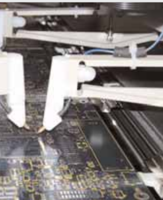
Netlist flying probe testing to reduce cycle time
