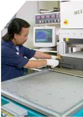
State-of-the-art continuous foil lamination press for controlled dielectric lamination
