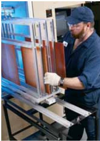
Plasma Chamber for precise etchback or desmear
